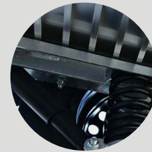
Hydraulic shock absorber
